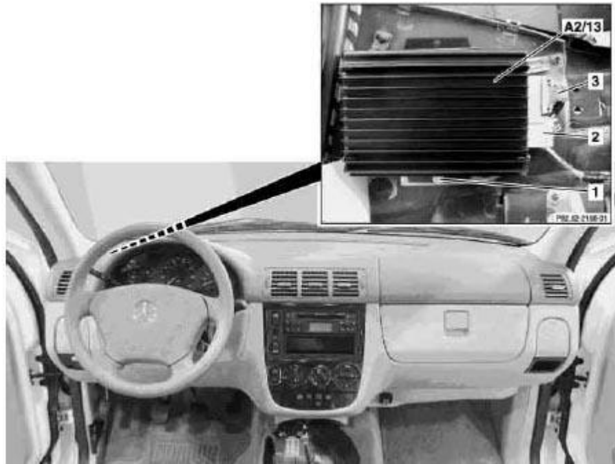
Fig. 195: Identifying Loudspeaker Amplifier Control Module Components
