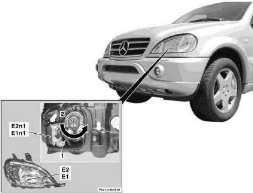
Fig. 159: Identifying Xenon Headlamp Control Unit Components
