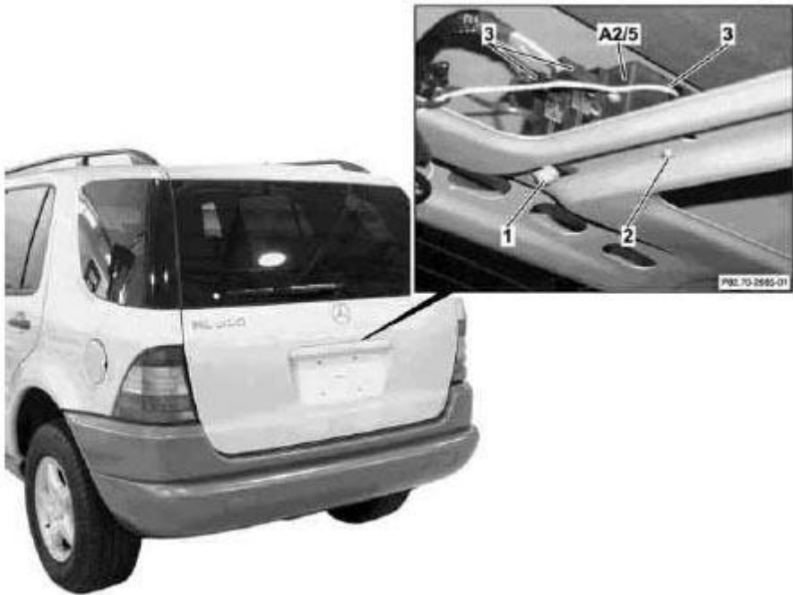
Fig. 216: Identifying Antenna Splitter Components
