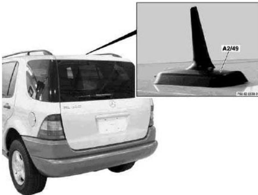
Fig. 77: Identifying CTEL And GPS Roof Antenna (01.09.01)
