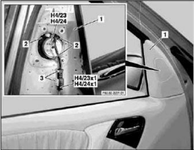
Fig. 199: Identifying Mirror Triangle Front Door Speaker Components
