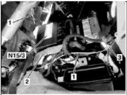
Fig. 204: Identifying ETC Control Module And Exchange D2B Wiring Harness
