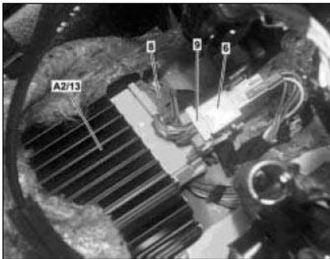
Fig. 100: Identifying Sound System Amplifier, Plug Male Connector A/B And Integrated Harness Clip
