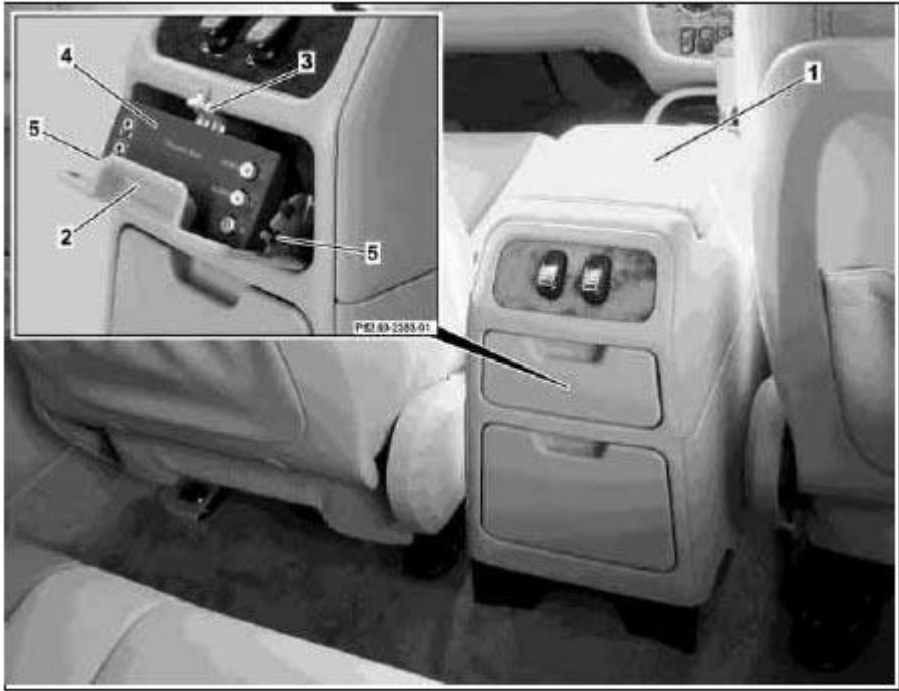
Fig. 299: Identifying Center Console, Auxiliary Interface Module And Retaining Spring
