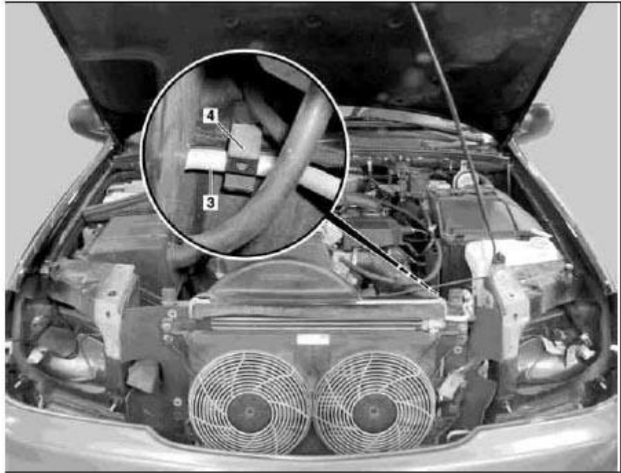
Fig. 188: Identifying Air Conditioning System Hose And Clip
