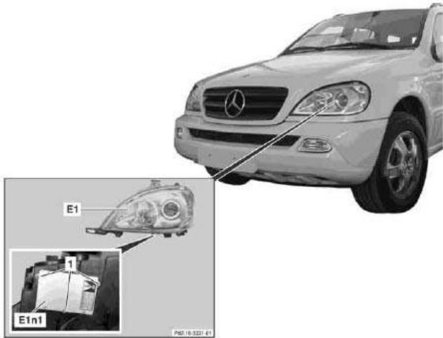
Fig. 161: Identifying Xenon Headlamp Control Unit Components
