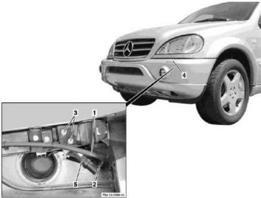
Fig. 171: Identifying Headlamp Cleaning System Components
